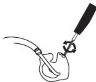
Cleaning the vent
