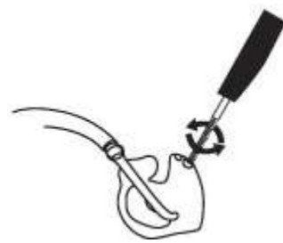
Cleaning the vent
